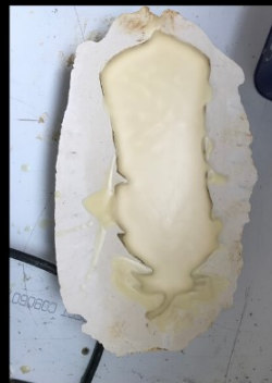
Plaster mould no.1 with wax setting in it.
