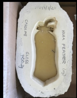
Plaster mould no.2 with waxed waiting to be steamed out
