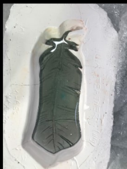
Glass inside mould no.2 after being fired in kiln.
