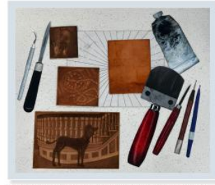
Mezzotint rocker, scraper, burnisher, rocking template, partially rocked plate. Plates for 'Heller' and 'Wedding Exchange'. JH
